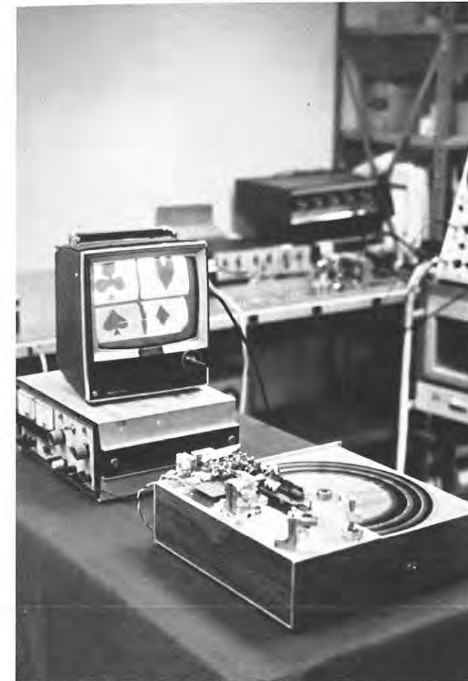
Figure 8. The video frame presented on the monitor is constructed from four different data tracks on the disc. There is one read-head (photodiode) per track, with an electronic switch between tracks effected twice per line and twice per field.
