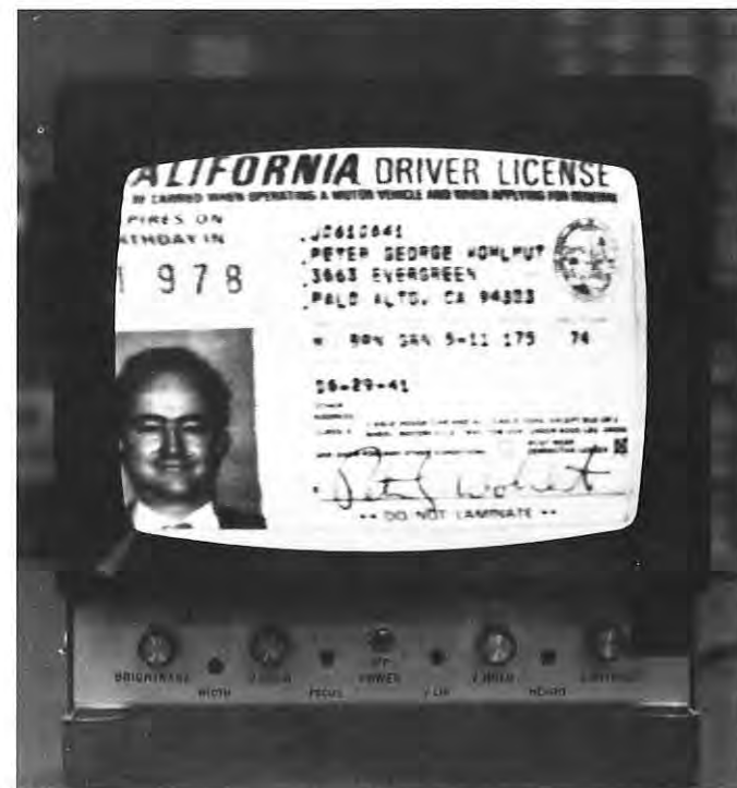
Figure 7. The video frame presented on the monitor is derived from a video player using a film disc and an incandescent source for illumination.
